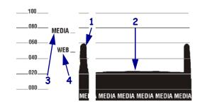
Figure 43 • Sensor Profile (Media Section)
